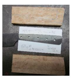
Shim stock can be used but so can old business cards (~0.010" thick). The appropriate number of thicknesses are positioned at the front spine and rear spine locations and the vise is closed. The end mill is positioned at the front spine location and the depth is set to  $\frac{1}{2}$  of the thickness of the tang at that location. Here that is 184, so 100 ought to do. Note that I round up a bit, usually 5 to 10 thousands. Afterall, the epoxy has to go somewhere.
