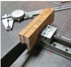
It is now glue time. You will need gloves, masking tape, 5-minute epoxy, epoxy colorant, 2 alignment pins and three C-clamps. The colorant I use came from Brownell's but is no longer available. A quick web search turned up "Castin' Craft Opaque Pigment 1 Oz: Black" which might do or even laser toner could suffice (if you can control that stuff!).
