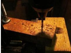
ream out the holes with a 0.125" bit. This process reduces the possibility of a pin hole being "wallowed" out and provides a tighter fit of pin to
